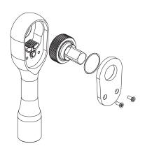
3. Pull on square end of gear to remove gear, o-ring and cover plate from the handle
