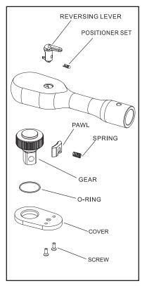
7. Replace cover plate and use star head driver to fasten plate screws.
