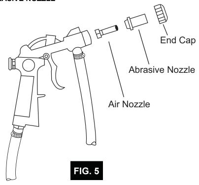
**IMPORTANT:** Be sure the air supply is disconnected before performing this operation.
