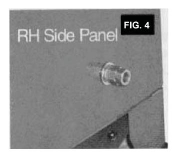
The air supply should be dry and capable of delivering a minimum of 10 CFM at 100 lbf/in2.
