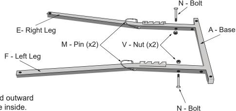
**NOTE:** The two legs must be angled outward with angle adjustment notches on the inside.
