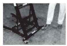
Lock Casters by pressing downward on the locking tab with your foot.
