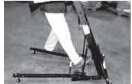
Push the Angle Adjustment Bar forward to the first setting of the notched Angle Adjustment Keeper.
