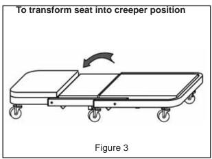
Step 3. Unlock the spring loaded Lock Pin by pulling out until disengaged, then reverse steps 1, 2 to convert Creeper Seat into Creeper.
