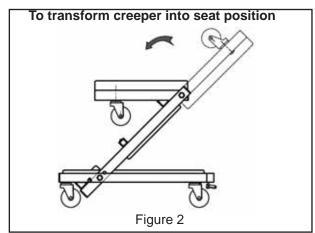
Step 1. Locate, then unlock the spring loaded Lock Pin by pulling out until disengaged, at the same time flip the Head Frame and Middle Frame upward and back towards the Rear Frame section until the Lock Pin can engage the Creeper Seat Locking Sleeve (Fig. 3). Ensure Lock Pin is fully engaged.
