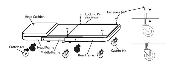
Figure 1 - Model ATD-81045 Components
