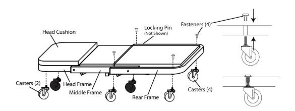
Figure 1 - Model ATD-81045 Components
