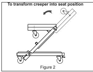
Step 1. Locate, then unlock the spring loaded Lock Pin by pulling out until disengaged, at the same time flip the Head Frame and Middle Frame upward and back towards the Rear Frame section until the Lock Pin can engage the Creeper Seat Locking Sleeve (Fig. 3). Ensure Lock Pin is fully engaged.
