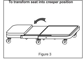
Step 3. Unlock the spring loaded Lock Pin by pulling out until disengaged, then reverse steps 1, 2 to convert Creeper Seat into Creeper.
