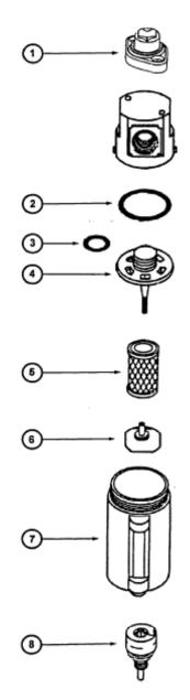
NOTE: Optional Automatic Float Drain is used for pressure from 30 psi to 175 psi, and from 40°F to 120°F
