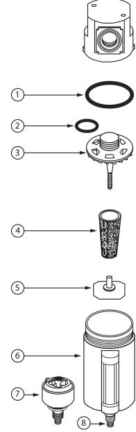
**Model 5200 Internal Float Drain Available (Item #7)** To be used for pressures from 30 psi to 175 psi and from 40°F to 120°F. To order filter with float drain assembled, add suffix "F" to filter model number.
