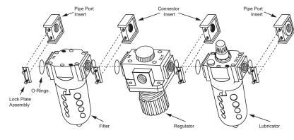
This exploded view drawing illustrates the engineering uniqueness of the modular system. Components shown can be ordered as a total system, or as individual items.
