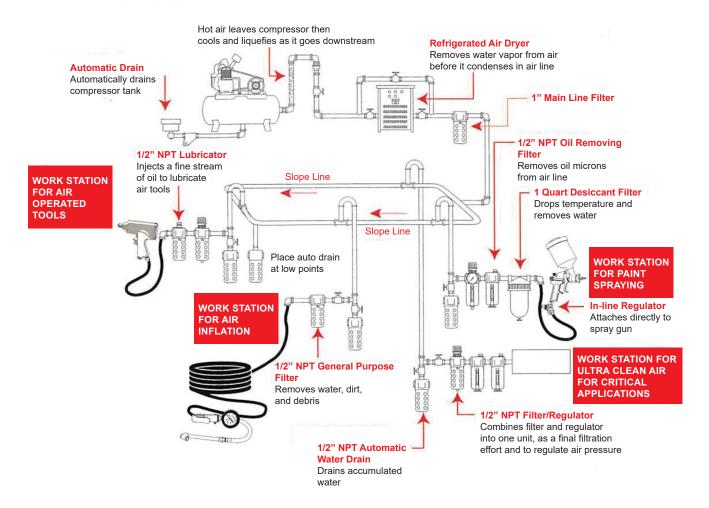
Compressed air powered equipment and machinery are critical elements in the productivity, efficiency and economy of today's industry, and quality air is the essential ingredient. Water and dirt cause more problems in compressed air lines than anything else. A typical 7.5 HP compressor brings an average of 3 gallons of water from the atmosphere per day along with dust and dirt in the air. It is important to eliminate water and dirt from your air system.
