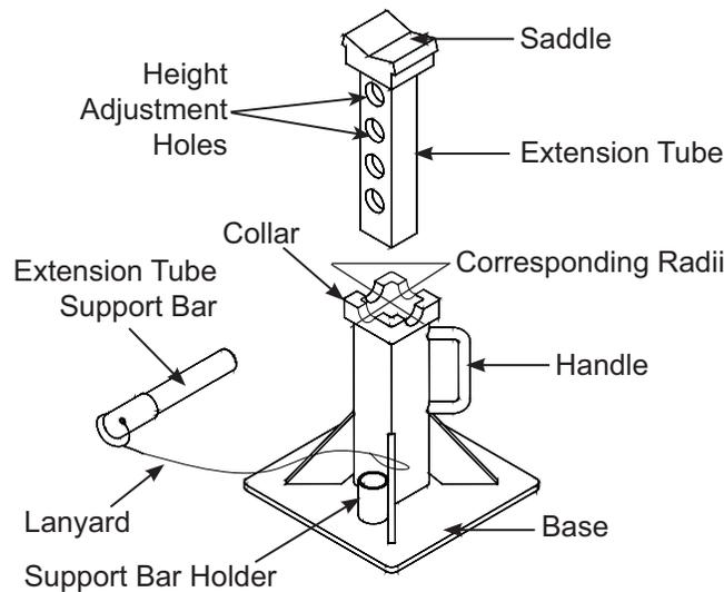
Figure 1 - Model ATD-7449A components
