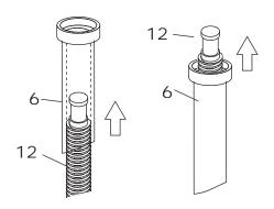
Install the Bearing (#5) by sliding it over the Extension Screw (#12) that is extended through the top end of the Column Tube (#6) until it seats into the flange at the top end of the Column Tube (#6). Make sure that the Bearing (#5) is between the two bearing washers and that the grooves in the washers are facing the bearing.
