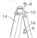
6. Slide Column Tube Assembly through connecting plate (#10) and Lower Plate (#11). Use Lock Pin and Chain assembly (#7) to lock tube in position.
