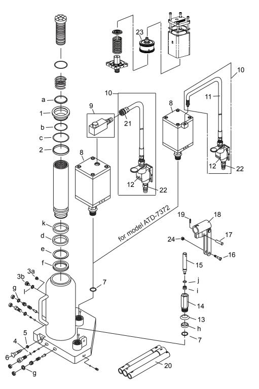
Figure 2 - Replacement Parts Illustration for Model ATD-7370, ATD-7371, & ATD-7372
