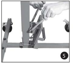
Attach support plate assembly to jack assembly (17) using 5/16" x 3 1/4" bolt. Note: do not over tighten.
