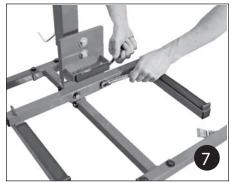
Attach support arm (14) to support plate assembly using 5/16" x 2" bolts. Tighten with 9/16" box wrench.
