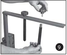
Attach vertical supports (2) using plastic knobs (1).
