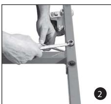
Insert support tube (11) into lower frame support (12). Tighten with wrench.
