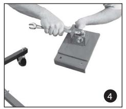
Bolt front support plate (3) to rear support plate (5) using 1/2" x 5/8" bolts and 1/2" lock nut. Note: do not over tighten.
