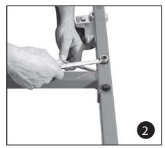
Insert support tube (11) into lower frame support (12). Tighten with wrench.
