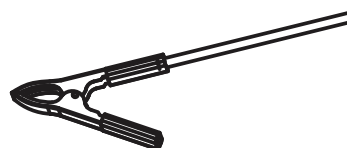
Ground Wire (yellow and green)
