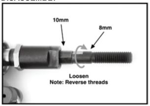
Use the provided wrenches or a 10mm and 8mm wrench to loosen the mandrel from the tool by turning it clock-wise due to the reverse threads.
