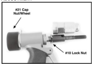
Adjustment of the stroke may be necessary at times based on the users application, however make sure the #10 Lock Nut is adjusted enough forward (and not too far back) so that the #4 connector housing relieves enough spring pressure when installed to allow the #21 Cap Nut/Wheel to freely spin. If the rear spinning wheel does not spin freely, adjust the #10 lock nut and #7 Spindle Guide until it does move freely with the #4 housing installed.
