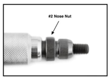
Install the #2 Nose Nut on each new nosepiece to be used. Adjust to lock the nosepiece in place closer or further away as needed. The further away from the tool the nosepiece is locked into place, the more the stroke will be applied to the rivet nut and/or the less the rivet nut can be threaded onto the mandrel.
