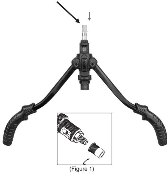
2. Insert the rivet nut into the pre-drilled hole in your workpiece after screwing the rivet nut to the mandrel. (Figure 2)
