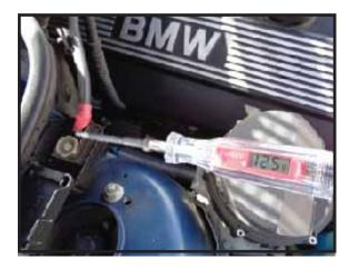
For smaller circuits where exacting precision is required, you can use a precision screwdriver or similar tool as a ground probe, connecting the ground to the end of the probe, while using the probe as the positive lead.
