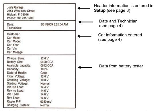
**NOTE**: To properly test the Electrical System (Full Test) the test sequence should be Battery Test, Starter Test, and then Charging System Test. The battery must be in good condition to properly test the Starter and Charging system. Therefore, the Starter Test Data and/or Charging Test Data may not show on the printout if either test is skipped.
