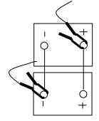
2- 12V batteries in parallel: add rated capacities of single battery. Pack is still 12V.
