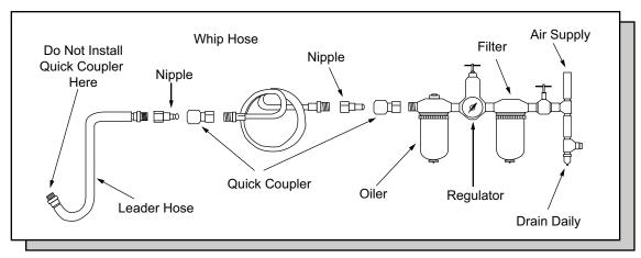
Always use clean, dry air. Dust, corrosive fumes and/or water in the airline will cause damage to the tool. Drain the air tank daily. Clean the air inlet filter screen on at least a weekly schedule. The recommended hook up procedure can be viewed in the above diagram.
