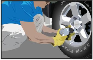
Remove lug nuts with an impact wrench, as you normally would. Remove the tire and wheel from the vehicle.
