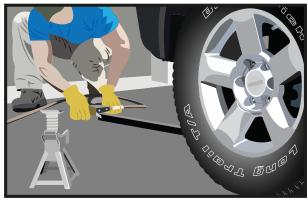
Lift the vehicle with jack in preparation to remove the tire. Secure the vehicle with stands or other approved equipment.
