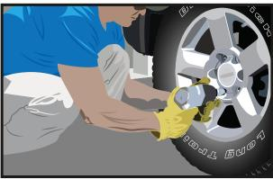
Replace wheel onto the hub and tighten all lug nuts to factory specifications. Raise vehicle off of jack stands (if applicable), remove stands, lower vehicle and the process is complete.
