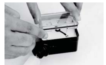
Place the needle back on the center pin, ensure that at the top most level the float and the needle is on the max. marking. Now close the lid.
