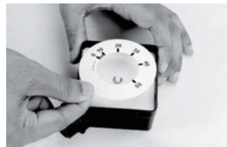
Flip the scale to switch between gallons/ liters. Align marking with the diagonal of the body.
