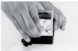
Open the cover of the indicator with the help of the notches provided on the sides
