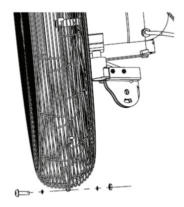
10. Secure the assembly of front and rear guards by tightening a screw and nut through the hole at the bottom position of the guards.
