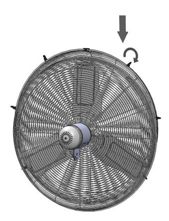
9. Assemble front guard to rear guard by fixing both guards together with clips on the rim of front guard positioning the hole in the guard rim at the bottom to match that of the rear guard.
