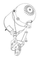
This fastening situation is for **Oscillation** operation.
