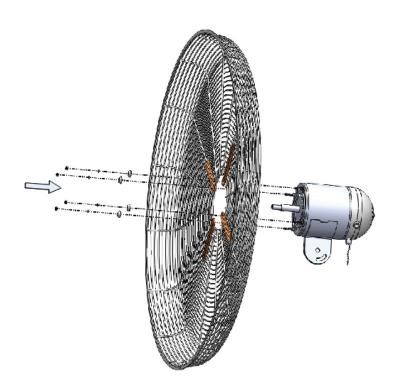
7. Set rear guard in proper position, with hole in guard frame at the bottom, and fix it to motor by securing with the hex nuts, spring washers and bowl washers that you removed in step 6.
