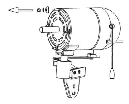
6. Remove four sets of hex nuts, spring washers and bowl washers from motor. Save them for step 7.
