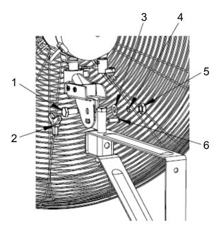
11. Insert the swivel plate into motor frame bracket and fasten it with #1, #3, #4 and #5 fasteners as shown above. Fasteners #2 and #6 will be used for adjusting the tilt angle of the fan.
