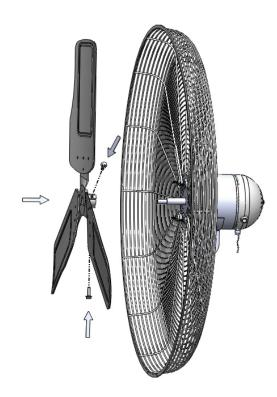
8. Assemble fan blade onto motor shaft by tightening the two screws. Make sure the screws are secured tightly.
