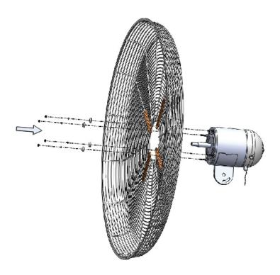
6. Set rear guard in proper position, with hole in guard frame at the bottom, and fix it to motor by securing with the hex nuts, spring washers and bowl washers that you removed in step 5.
