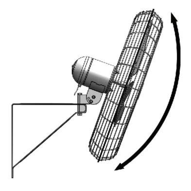
11. To adjust tilt of fan, loosen nut and bolt assembly in the slotted hole, tilt fan to desired angle and tighten nut and bolt assembly to secure.
