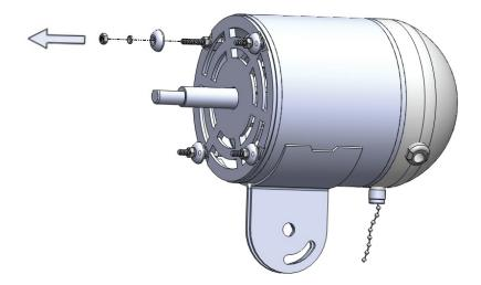
5. Remove four sets of hex nuts, spring washers and bowl washers from motor. Save them for step 6.
