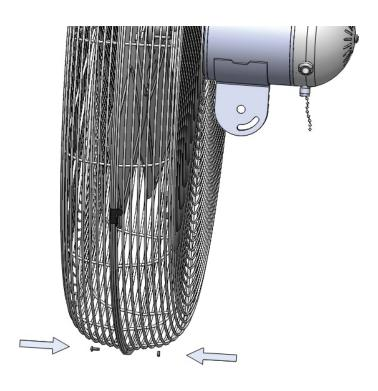
8. Secure the assembly of front and rear guards by tightening a screw and nut through the hole at the bottom position of the guards.
