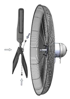
7. Assemble fan blade onto motor shaft by tightening the two screws. Make sure the screws are secured tightly.
