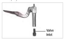
10. Take out the cylinder (9) containing ball spring (8) and ball retainer (7) carefully.
