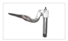
14. Pull out the piston (22) from the top of the grease control valve.
