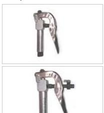
21. Thread tighten the extension (24) and grease coupler (23) onto the valve outlet (16).
