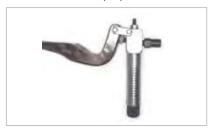
20. Bring back the handle (18) to the original position and fix it in place
