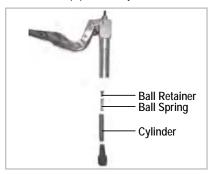
11. Tap the grease control valve on the floor from the bottom side to take out the steel ball (1/4") (6).
