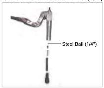
12. Replace the old steel ball (1/4") (6), ball spring (8) and ball retainer (7) with the new ones from the repair kit.
