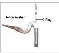
17. Replace the old parts with new parts (piston, rod guide, Teflon washer, O-Ring) from the repair kit.
