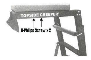
ATTACH BUMPER PADS To angle adjustment bars and adjustment pin cross bar as shown
