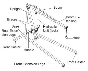
Figure 1- Model Atd-7484 Components
