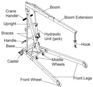
Figure 2- Model Atd-7485 Components
