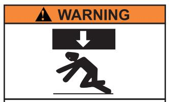
To avoid crushing and related injuries: NEVER work on, under or around a load supported only by engine crane. Immediately transfer the load to an appropriately rated engine stand.
