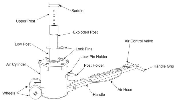
Figure 1 - Air Jack/Support Stand Components
