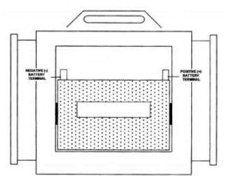
FIGURE 2. - REAR VIEW OF THE POWER PACK UNIT SHOWING THE BATTERY COMPARTMENT
