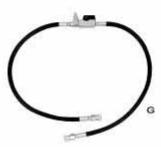
G.— CIS/TBI Test Hose - use when testing CIS or TBI Systems where in line connections are needed.Includes shut-off valve for both control & primary system pressure checks.We recommend that the D Gauge Hose is used with CIS testing, as most manufacturers require that all air be purged from the tester when running tests.
