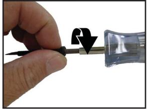
The small and large alligator clips slide onto the adapter, then into the circuit tester handle as shown below.
