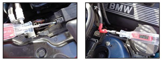
For smaller circuits where exacting precision is required, you can use one probe as a ground probe, connecting the ground to the end of the probe, while using the other probe as the positive lead.
