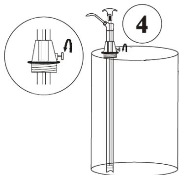
4. Now **very lightly** tighten the bung onto the pump tube. Note that excessive tightening may damage the pump & render it inoperative.
