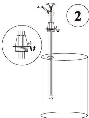
2. Loosen the bung nut fitted onto the pump tube & insert the pump into the drum from the 2" threaded opening on the drum.
