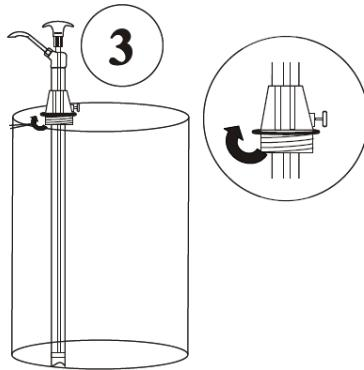
3. Once the bottom of the pump touches the base of the drum, securely fasten the bung onto the drum.
