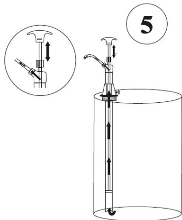
5. Take an empty container & place it below the discharge spout. Start operating the pump handle by moving it up by about 12" & then down. Within a maximum of 4 strokes, pump will be primed & will start dispensing media. Amount of fluid discharge per stroke can be controlled by the lift of the pump handle. The more it is lifted, the greater will be discharge per stroke. Never take the pump handle to its extreme top position, but operate within a convenient lift height.
