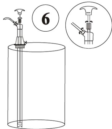
6. There maybe some leakage of media from the plunger rod guiding nut. The nut is factory tightened for test media. Depending upon the viscosity of media used, the nut should be loosened or tightened to control any flow of media from this connection. Also, you may need to slightly adjust the Threaded Nut, if there is any leakage from this connection.
