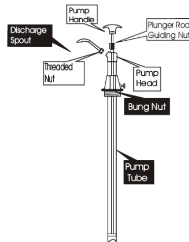
1. Assemble the Discharge spout onto the pump head, using the threaded nut fitted onto the spout. Tighten the connection by hand. Do not over tighten, as you may strip the threads.
