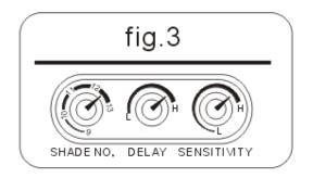
the mask is disturbed by excess ambient light or another welding machine close by, use the "low" setting. (See fig.3)
