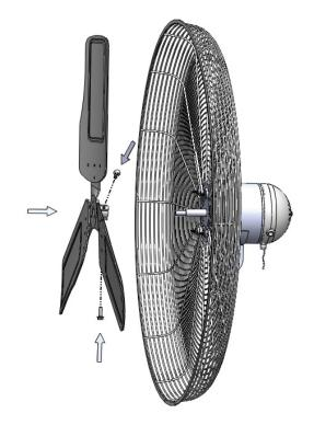
8. Assemble fan blade onto motor shaft by tightening the two screws. Make sure the screws are secured tightly.
