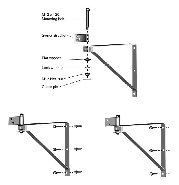
**CAUTION:** This fan is only suitable for mounting in studs or in a concrete wall. Do not use on dry wall, or other hollow wall mounting. Use the mounting accessories shipped with products for wall mounting.
