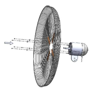
7. Set rear guard in proper position, with hole in guard frame at the bottom, and fix it to motor by securing with the hex nuts, spring washers and bowl washers that you removed in step 6.
