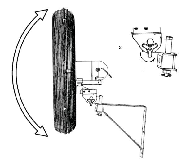
12. Loosen #2 as mentioned in step 11, to change the tilt angle of the fan.
