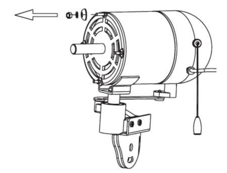
6. Remove four sets of hex nuts, spring washers and bowl washers from motor. Save them for step 7.
