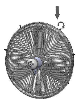
9. Assemble front guard to rear guard by fixing both guards together with clips on the rim of front guard positioning the hole in the guard rim at the bottom to match that of the rear guard.
