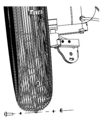
10. Secure the assembly of front and rear guards by tightening a screw and nut through the hole at the bottom position of the guards.
