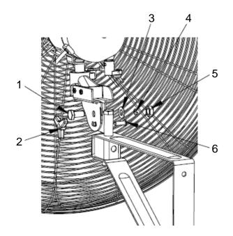
11. Insert the swivel bracket into motor frame bracket and fasten it with #1, #3, #4 and #5 fasteners as shown above. Fasteners #2 and #6 will be used for adjusting the tilt angle of the fan.
