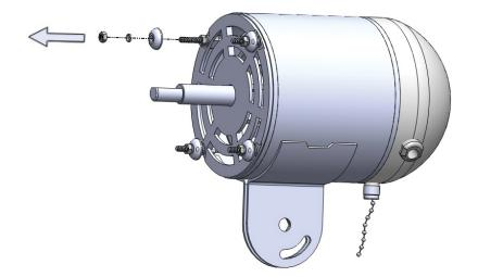
5. Remove four sets of hex nuts, spring washers and bowl washers from motor. Save them for step 6.
