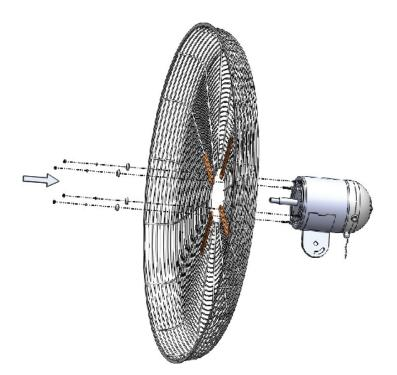
6. Set rear guard in proper position, with hole in guard frame at the bottom, and fix it to motor by securing with the hex nuts, spring washers and bowl washers that you removed in step 5.
