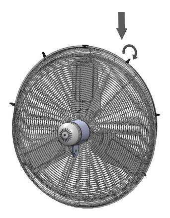
7. Assemble front guard to rear guard by fixing both guards together with clips on the rim of front guard positioning the hole in the guard rim at the bottom to match that of the rear guard.
