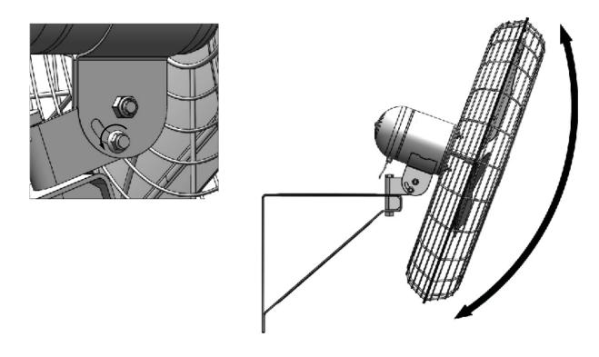
11. To adjust tilt of fan, loosen nut and bolt assembly in the slotted hole, tilt fan to desired angle and tighten nut and bolt assembly to secure.
