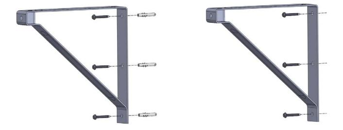
**CAUTION:** This fan is only suitable for mounting in studs or in a concrete wall. Do not use on dry wall, or other hollow wall mounting. Use the mounting accessories shipped with products for wall mounting.
