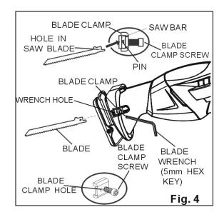
3. Align the hole in the shank of the blade and blade clamp with the pin in the saw bar, and then seat both on the pin in the saw bar.
