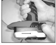
**CAUTION:** When placing battery pack in your cordless impact wrench, be sure raised rib on battery pack aligns with groove in wrench's battery port and latches snap in place properly. Improper assembly of battery pack can cause damage to internal components.
